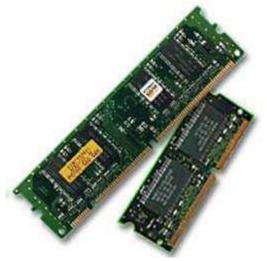
The word **static** indicates that the memory retains its contents as long as power is being supplied. However, data is lost when the power gets down due to volatile nature. SRAM chips use a matrix of 6-transistors and no capacitors. Transistors do not require power to prevent leakage, so SRAM need not be refreshed on a regular basis.
