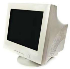
A finite number of characters can be displayed on a screen at once. The screen can be divided into a series of character boxes - fixed location on the screen where a standard character can be placed. Most screens are capable of displaying 80 characters of data horizontally and 25 lines vertically.
