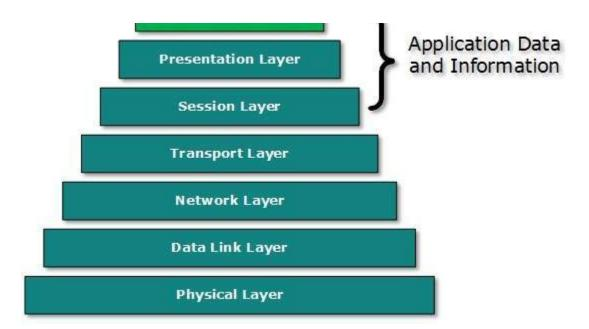
There'is an ambiguity in understanding Application Layer and its protocol. Not every user application can be put into Application Layer. except those applications which interact with the communication system. For example, designing software or text-editor cannot be considered as application layer programs.
