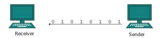
Serial transmission can be either asynchronous or synchronous.
