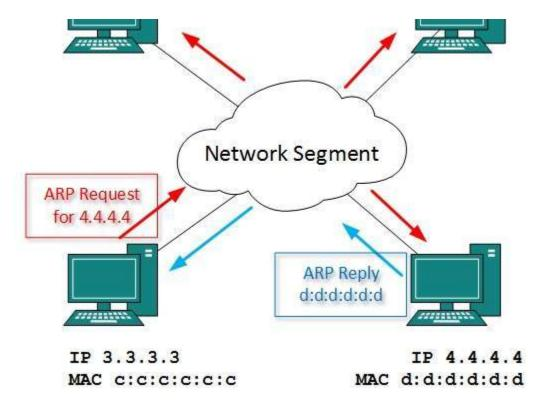
To know the MAC address of remote host on a broadcast domain, a computer wishing to initiate communication sends out an ARP broadcast message asking, "Who has this IP address?" Because it is a broadcast, all hosts on the network segment *broadcastdomain* receive this packet and process it. ARP packet contains the IP address of destination host, the sending host wishes to talk to. When a host receives an ARP packet destined to it, it replies back with its own MAC address.
