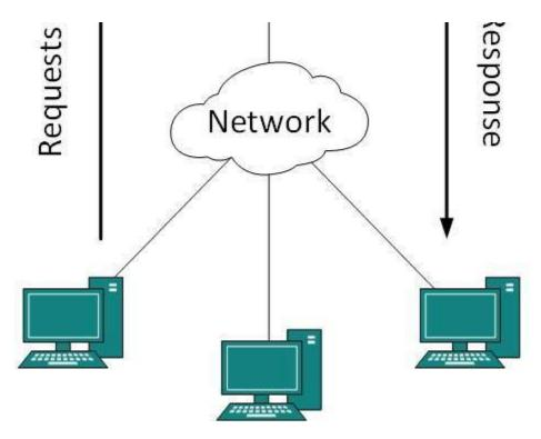
A system can act as Server and Client simultaneously. That is, one process is acting as Server and another is acting as a client. This may also happen that both client and server processes reside on the same machine.
