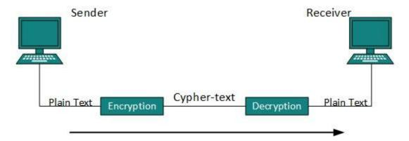
Cryptography is a technique to encrypt the plain-text data which makes it difficult to understand and interpret. There are several cryptographic algorithms available present day as described below:
