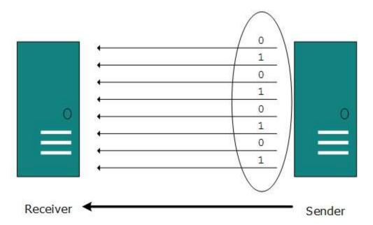
The binary bits are organized in-to groups of fixed length. Both sender and receiver are connected in parallel with the equal number of data lines. Both computers distinguish between high order and low order data lines. The sender sends all the bits at once on all lines. Because the data lines are equal to the number of bits in a group or data frame, a complete group of bits data frame is sent in one go. Advantage
