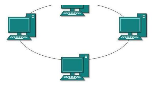
Failure of any host results in failure of the whole ring. Thus, every connection in the ring is a point of failure. There are methods which employ one more backup ring.
