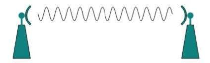
Microwave antennas concentrate the waves making a beam of it. As shown in picture above, multiple antennas can be aligned to reach farther. Microwaves have higher frequencies and do not penetrate wall like obstacles.
