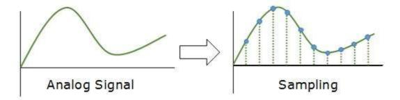
The analog signal is sampled every T interval. Most important factor in sampling is the rate at which analog signal is sampled. According to Nyquist Theorem, the sampling rate must be at least two times of the highest frequency of the signal.
