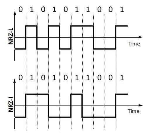
NRZ-L changes voltage level at when a different bit is encountered whereas NRZ-I changes voltage when a 1 is encountered.
