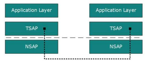
For example, when a DHCP client wants to communicate with remote DHCP server, it always requests on port number 67. When a DNS client wants to communicate with remote DNS server, it always requests on port number  $53\ UDP$ .
